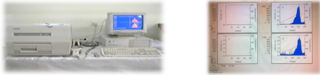
Figure 4. Dosimetric system for analyzing the data registered by dosimetric cards
