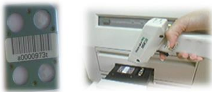
Figure 3. Dosimetric cards used to evaluate the dose
